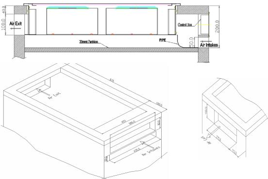
Control box cut off : 365(W) x 83mm (H) Air in-take cut out: 435mm (W) x 50mm (H) Air exhaust cut out: 275mm (W) x 100mm (H) 22 Sept., 2003
